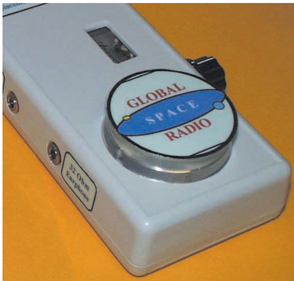
The translucent "furniture cup" is held in position on the case by the sounder mounting lugs.
